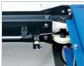
Electric height-limit switch provides safekeeping of the vehicle during lifting.
